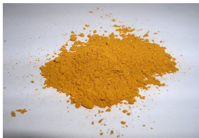
Fig. 2 One gram of V_2O_5 nanorod powder obtained after 5 min of annealing in a fluidized (vibrating) bed at 600 °C
